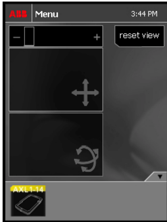
Figure 4: A screenshot from the interface presented to the user on the personal mobile device when in front of the ABB Powerwall. The interface widgets for controlling and manipulating the currently active object (AXL1-14) are the same on the personal device as they are on the large, shared display.
