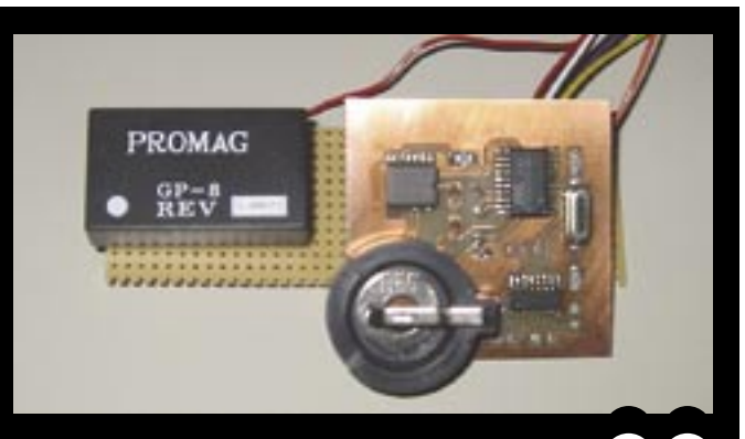
Figure 1. The custom made hardware required for the prototype implementation. The RFID tag reader to the left, and the tilt sensor to the right, including battery holder and microprocessor
